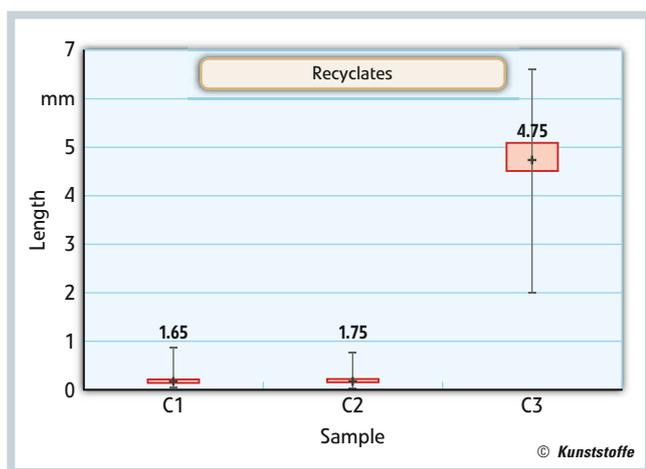
**Fig. 6. Length distribution of the short filaments with median values**
