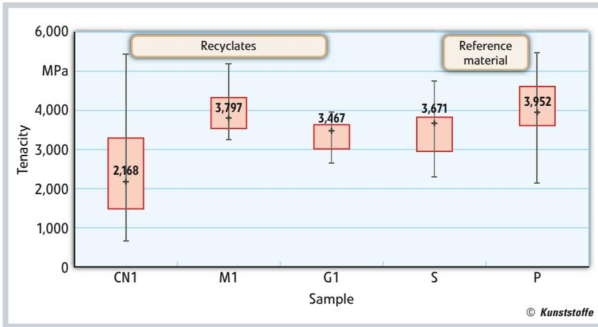
Fig. 3. Tenacity distribution of the roving snippets with median values
