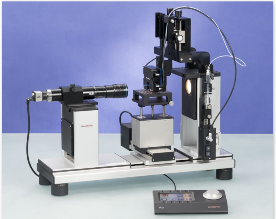
contact angle measurements on micro-structured samples using an OCA 200 with nanolitre and picolitre dosing systems
