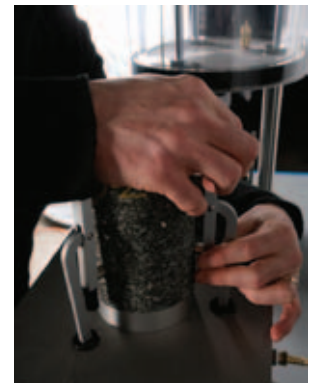
1. Place specimen in jig
