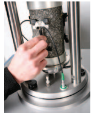
2. Mount strain transducers
